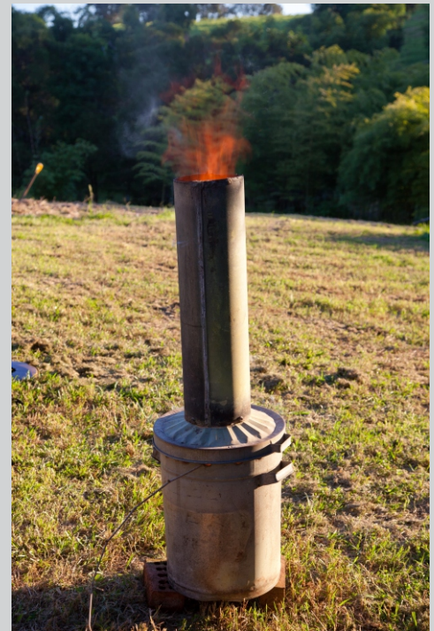
A TLUD burner producing a quality product Biochar.
