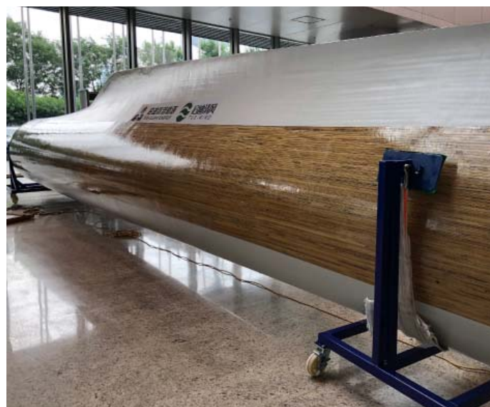
High tech bamboo wind turbine blades
