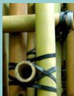
Left, Test frame with clothes. Right, the finished product. Below right, building the frames on a jig, lot of knots to tie. Below is a detail of the final tied bamboo.
